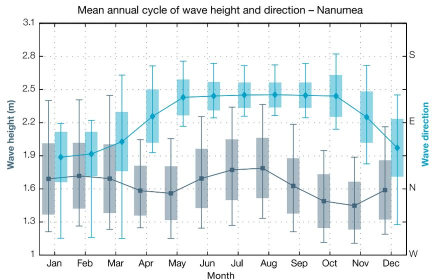
**Figure 4:** Annual cycle of wave height (grey) and wave direction (blue) at Funafuti (top) and Nanumea (bottom) based on data from 1979–2009. The shaded boxes represent one standard deviation around the monthly means, and the error bars indicate the 5–95% range, showing the year-to-year variability in wave climate. The direction from which the waves are travelling is shown (not the direction towards which they are travelling).
