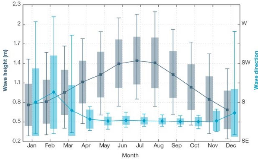
Figure 11.1: Mean annual cycle of wave height (grey) and mean wave direction (blue) at Port Moresby in hindcast data (1979–2009). To give an indication of interannual variability of the monthly means of the hindcast data, shaded boxes show 1 standard deviation around the monthly means, and error bars show the 5–95% range. The direction from which the waves are travelling is shown (not the direction towards which they are travelling).
