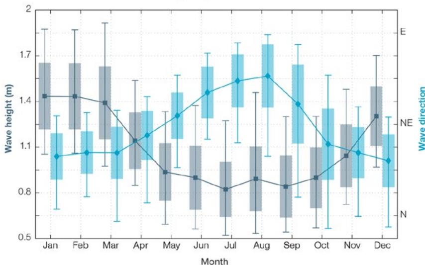
Figure 11.2: Mean annual cycle of wave height (grey) and mean wave direction (blue) at Kavieng in hindcast data (1979–2009). To give an indication of interannual variability of the monthly means of the hindcast data, shaded boxes show 1 standard deviation around the monthly means, and error bars show the 5–95% range. The direction from which the waves are travelling is shown (not the direction towards which they are travelling).
